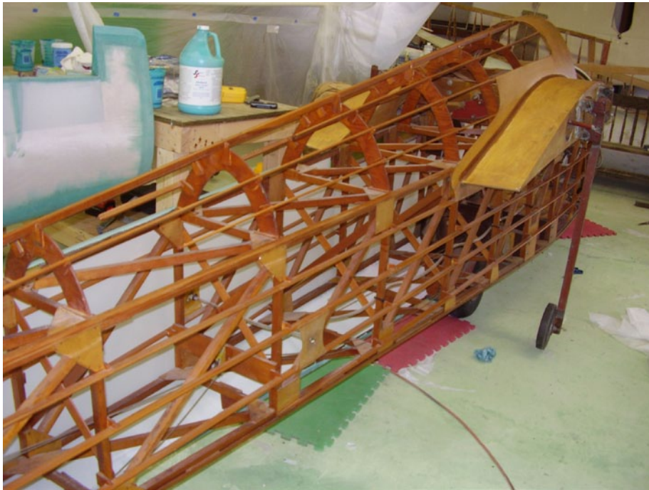
Right side of the fuselage skeleton, ready for covering.
