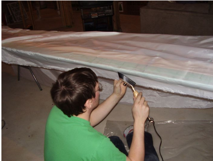
We glued three inches either side of the leading edge and along the root and tip and both side of the trailing edge. The fabric laid in place pretty well. We would heat the leading edge in place first and then work the top of the leading edge in place.
