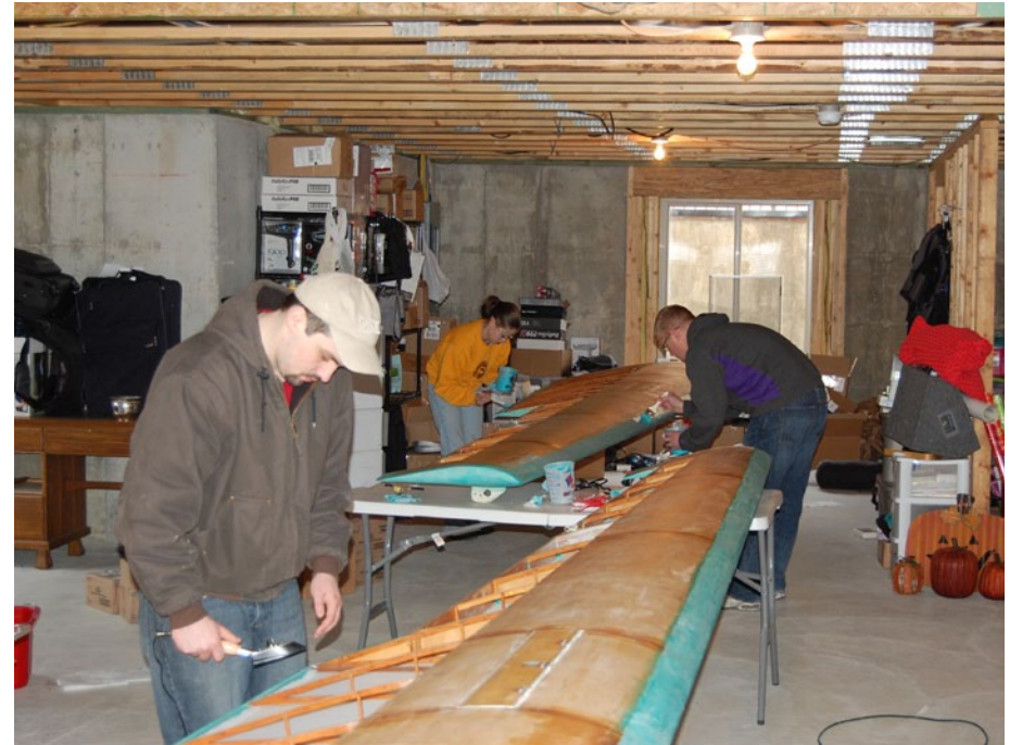
With the rest of the fabric blanket free to move there were very few issues with wrinkles. Then we'd attach the trailing edge, root, and tip. Then flip the wing over and do the top of the leading edge and the top of the trailing edge.
