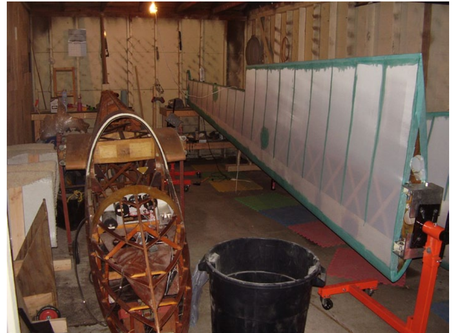
Another shot of the fuselage skeleton; left wing on the right.
