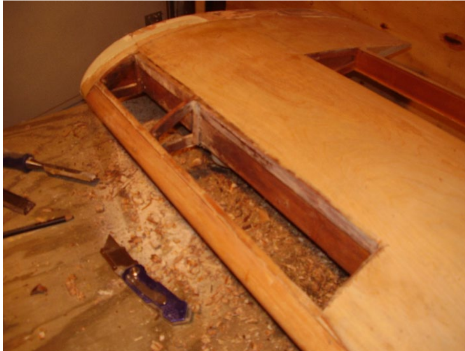
Rotten wood removed from the top surface of the right wing.
